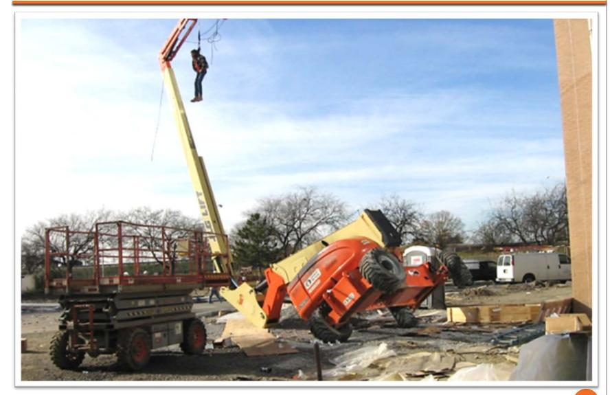
When using a fall protection harness and lanyard, using either a manufacturer approved, rated anchorage point or a heavy gauge steel guardrail is an approved method for tying off.
